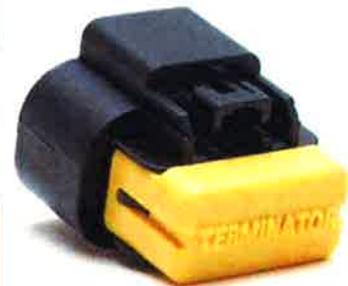
If using this 10-pin wiring, you will remove this cap and re-use this at your J-box location. A Blue Data cable with terminating resistor will plug into connector that was capped with the cap shown above. On the Blue Data Cables, the terminating resistor location will be indicated by the yellow band on the harness. Yellow band needs to go to engine connection.
