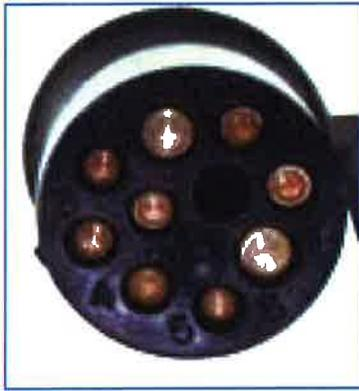
Determine what engine connector you have. If 10-pin you can only run Blue Data Harness for Smart Craft. If 14-pin the helm harness may have a SmartCraft 10-pin plug for Junction-Box or Gauge connection.
