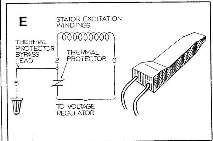
**IMPORTANT:** Note the thermal protector is connected in series with stator excitation winding output wire #2. In case of thermal protector failure, a BYPASS LEAD (Wire #5) is provided. To bypass a defective thermal protector, simply connect Wire #2 from the voltage regulator to Wire #5 using the supplied wire nut. When the thermal protector is bypassed, no generator overtemperature protection is available.
