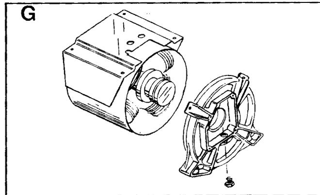
Retain REAR BEARING CARRIER and STATOR to BLOWER HOUSING with the four long STATOR BOLTS and LOCKWASHERS. Tighten STATOR BOLTS to 10-12 foot-pounds (14-16 N-m). Recheck flushness of STATOR CAN against REAR BEARING CARRIER and BLOWER HOUSING.
